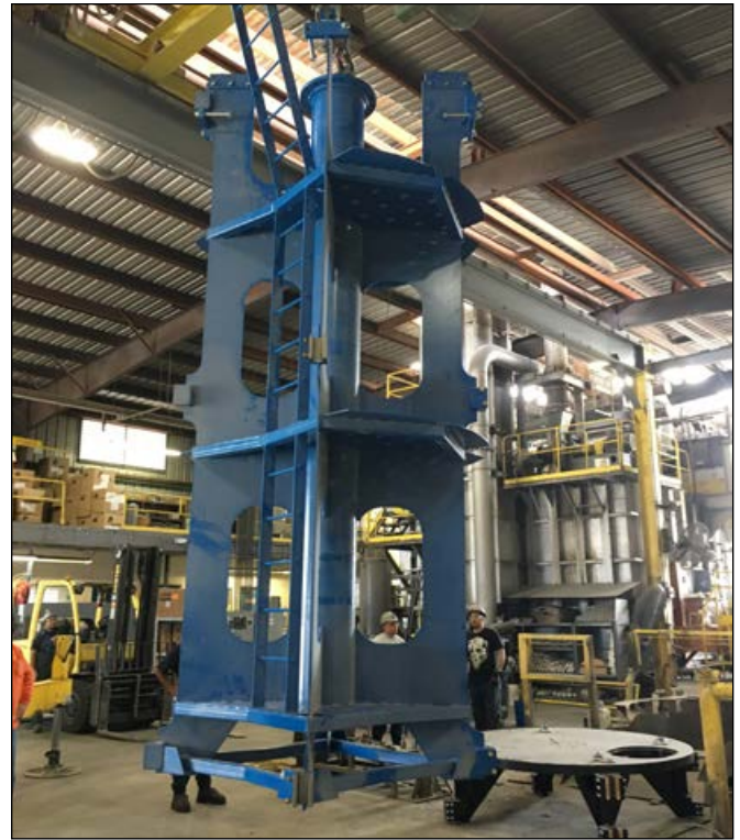
Figure 3. Full height jig fixture built for casting pit.
